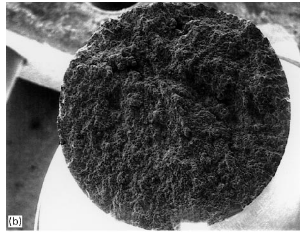
Figure 5 (a) SEM images of room temperature tensile fracture surface of a longitudinal sample. (b) SEM images of elevated temperature tensile fracture surfaces of longitudinal samples.
