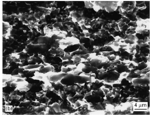
Figure 9 SEM images of tensile fracture surfaces of samples tested at 371 °C. (a) Longitudinal; (b) transverse.
